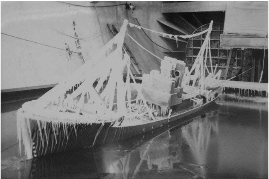
The model trawler, close to capsizing, in the Stratosphere Chamber at Weybridge
