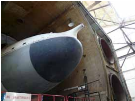
Preparing part of a Valiant fuselage for testing in the Stratosphere Chamber
