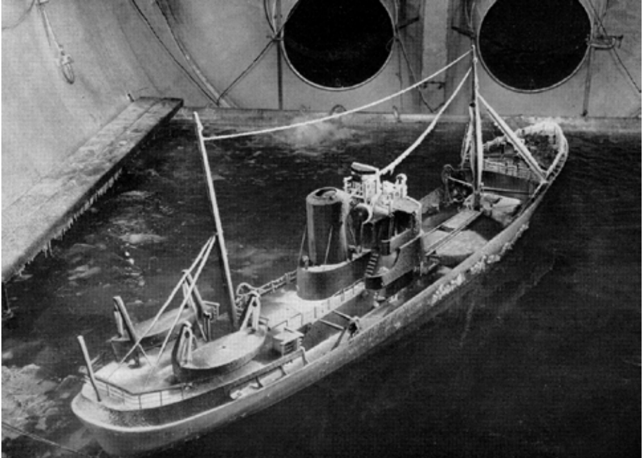
Fig.2. An 18ft model trawler begins its tests under icing conditions; as yet the layer is thin. Driving rain and blizzards can be produced if required.
