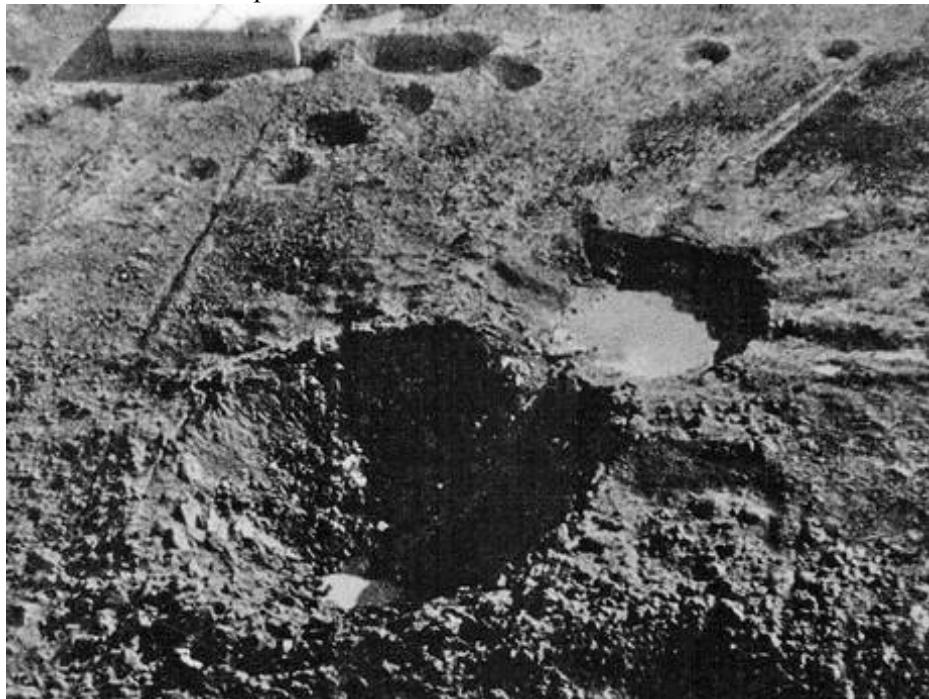
The 70 ft deep and 130 ft diameter crater which Grand Slam created in the New Forest on 13 March 1945 - with the target building in the background (Crown Copyright)
